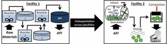
FIGURE 2. Continuous manufacturing efforts in the pharmaceutical industry vary significantly.
