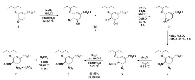
FIGURE 4. Current synthetic route of Oseltamivir Phosphate.
