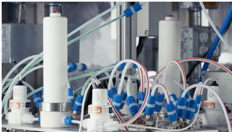
Fig. 4 Clarification Bypass Unit
