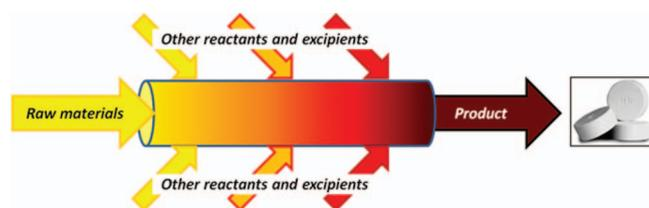
**FIGURE 3.** Concept of integrated continuous manufacturing of pharmaceuticals.
