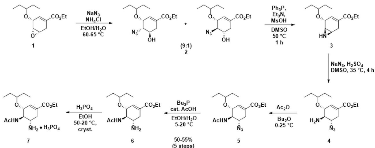
**FIGURE 4.** Current synthetic route of Oseltamivir Phosphate.
